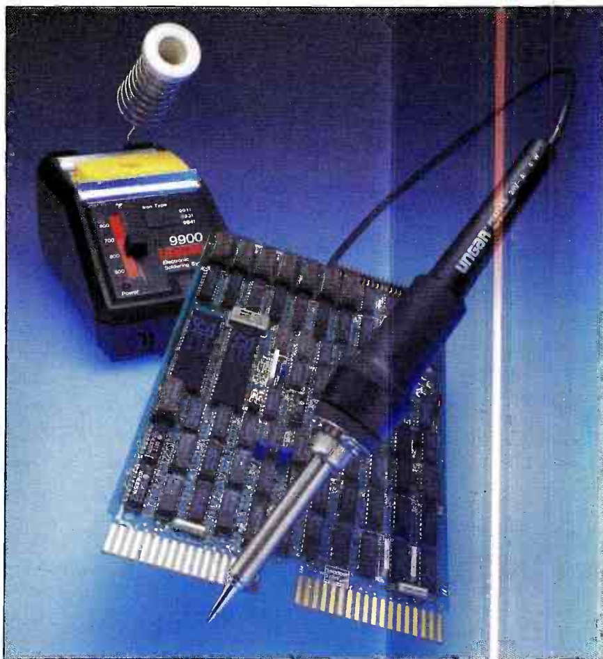
Successful solder rework of a printed circuit board requires skill, patience and the proper tools. One of those tools is a temperature-controlled soldering iron.
